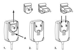
Fig. 1.1: Swapping plugs on the switching power supply unit
