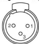
DMX - output XLR mounting-sockets (rear view):
